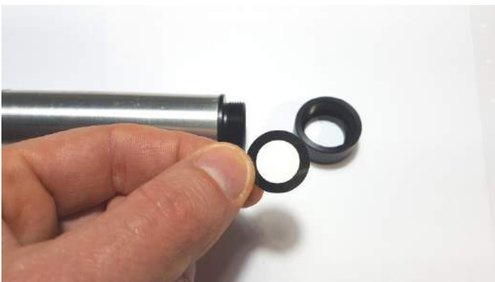
2 - Place the membrane Black ring face up
