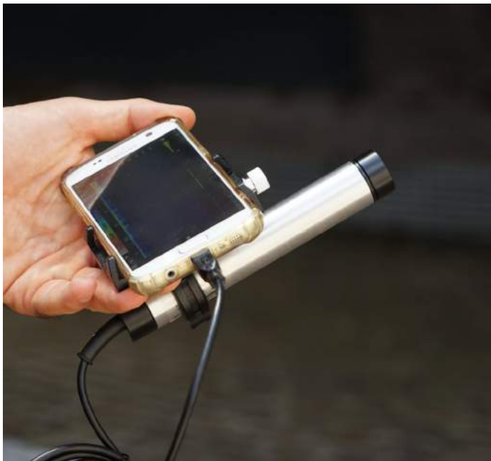
Smartphone and UM384K with the microphone metal holder.
