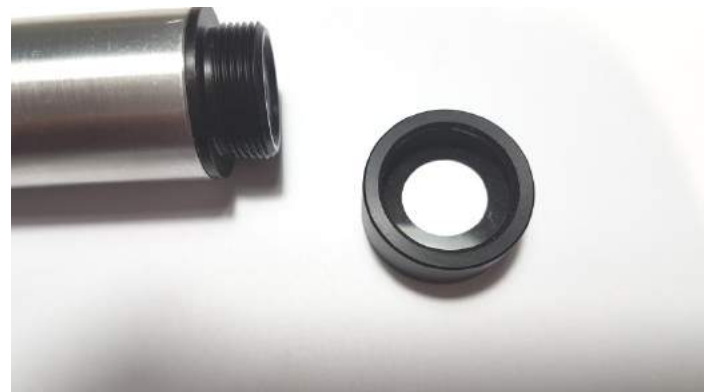
6 - The membrane can be easily unmounted unscrewing the top cap
